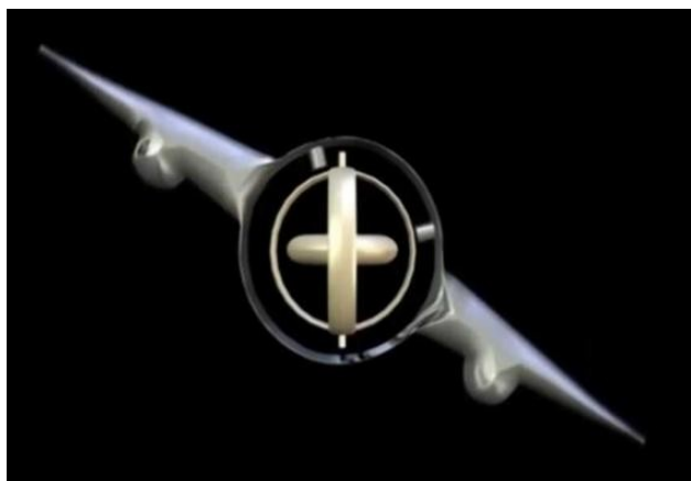
89. Plane tilted, gyroscope compensates
